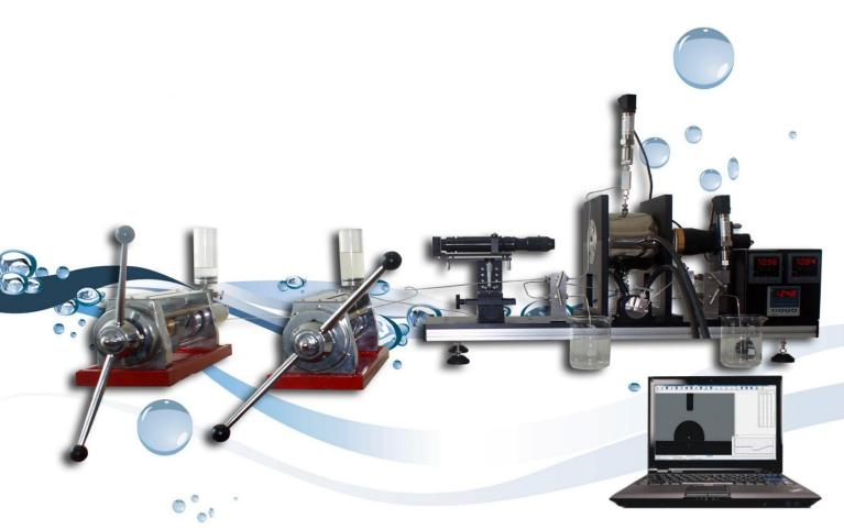
Drop shape analysis system model SL200HP is designed for measurement of contact angle, surface tension (liquid-gas) or interfacial tension (liquid-fluid) under such special conditions as ultra-high pressure (max 75Mpa) and high temperature (max 200°C). Thanks for its heating cell for such viscous sample as crude oil, SL200HP is the only instrument that can be used for application of tertiary oil recovery (EOR) especially for measurement of interfacial tension between ASP-crude oil.
